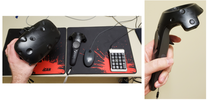
Fig. 4. The equipment for Study 1: HTC Vive headset and controller (held in the NDH), mouse (for the DH) and keypad (to advance to the next trial after a break).
