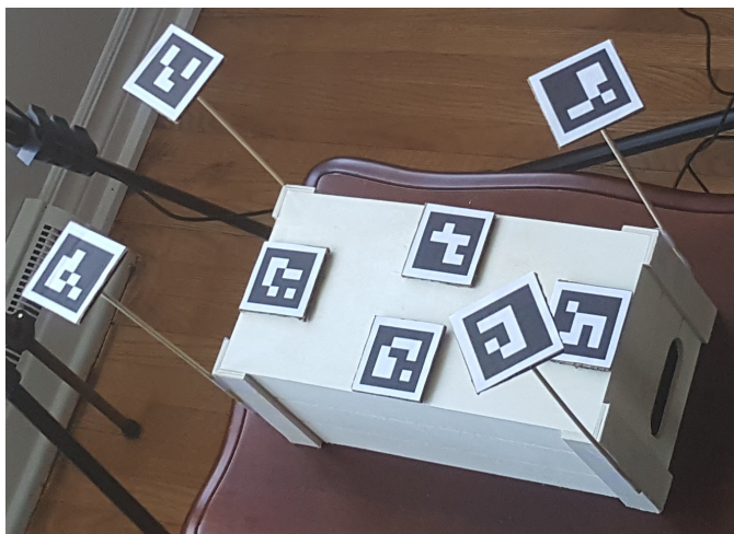
Figure 2: Registration rig with 8 fiducials.
