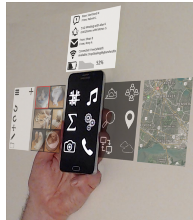
Figure 1: The extended space around the phone, displayed using augmented reality, is aligned to be co-planar with the phone’s physical screen. The extended space around a phone could display additional screens and running applications that the user can switch to (mock-up).
