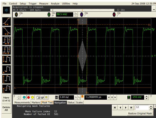
Figure 2: Screenshots from the GUI for a commercial oscilloscope. The oscilloscope’s GUI is operated with a mouse. Top : an eye diagram with a rhombus-shaped “mask” defined by the user. Traces that intersect the rhombus are classified as anomalies, in this case because they transition too late or too early. Bottom : the eye diagram is unfolded, and the user may jump forward or backward with buttons in the lower right to view each of the hundreds of anomalies within its local temporal context.
