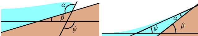
Figure 10: From contact angle \alpha and solid tilt angle \beta , we obtain the correction angle \psi to apply to the normal at the contact point
